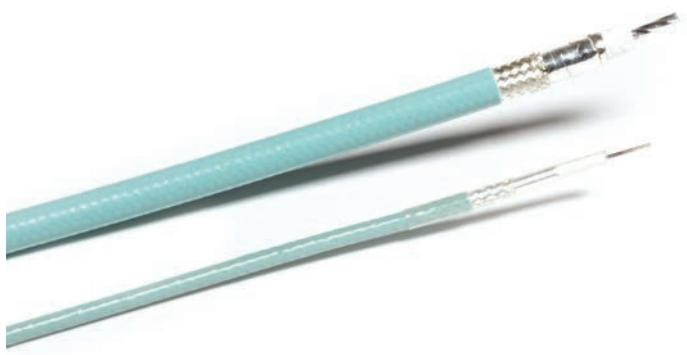
M-FLEX Microwave coaxial cables are a family of flexible cables designed to accept connectors designed for Semi-Rigid cable. Unlike other single or double braided "RG" type flexible cables, M-FLEX cables are true microwave cables capable of operating to frequencies of 26.5 GHz. The extended frequency range is the result of a precision helically wrapped silver plated copper foil inner shield. This inner shield allows for outstanding flexibility while providing 100% coverage.
