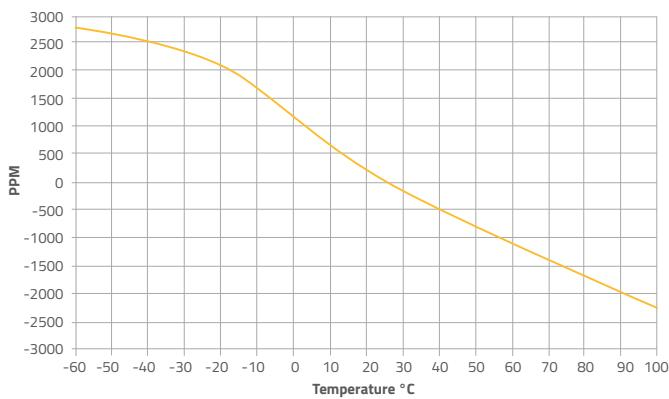
Typical Phase Change vs. Temperature Low Loss PTFE Cables
