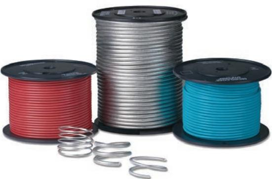
UTiFORM cables are hand-formable and are designed to the same dimensions as many standard Semi-Rigid cables. UTiFORM cables employ a tin soaked copper braid that is easily solderable and allows the cable to be reshaped many times. UTiFORM cables are available with and without an FEP insulating jacket and are supplied in long continuous lengths, which make them ideal for automated cutting and stripping equipment.
